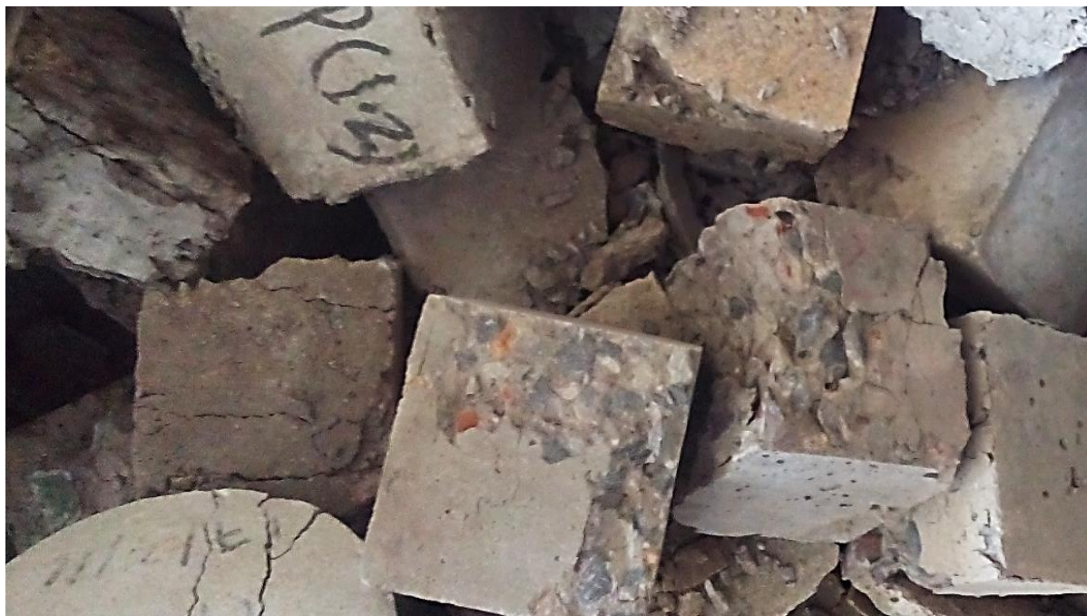
Fig. 1: Concrete Debris Aggregates.
