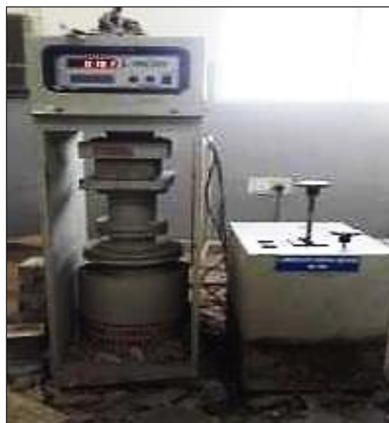
Fig. 4: Compression Test being carried out on Bricks Using a Compression Testing Machine.
