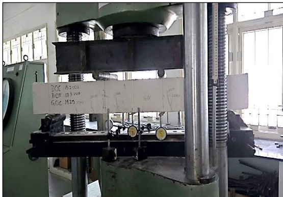
Fig. 8: Testing of Beam in UTM.
