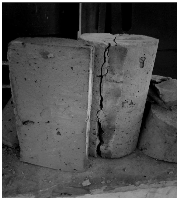
Fig. 2: Split Tensile Test.
